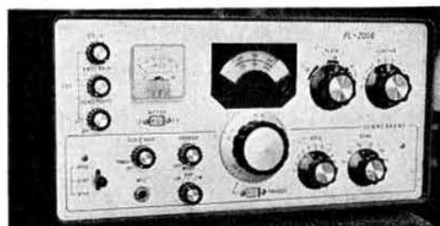
FL-200-B Tx. AM/CW/SSB. 240W p.e.p., 100W AM VOX, PTT, Break-in CW. Sidetone monitoring. Connectors for transceiver with the FR-100-B supplied. Note:—The 6JS6A finals are the same electrically as the 6HF5 so the power ratings are conservative. £130.
